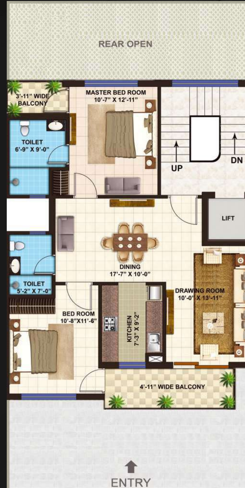
TYPICAL FLOOR PLAN (UPPER GROUND & FIRST FLOOR)
