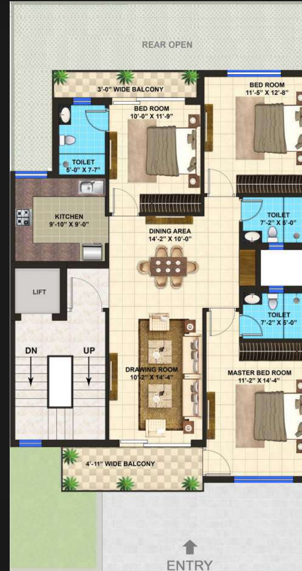
TYPICAL FLOOR PLAN (UPPER GROUND & FIRST FLOOR)
